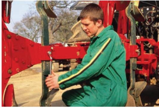
Before attempting any maintenance work on a machine, make sure the machine is safe to work on by following the Safe Stop procedure.
